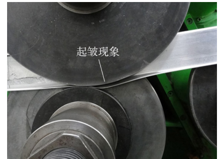
图6 Z型材下缘板失稳起皱 Fig.6 Wrinkling of Z-shaped profiles during roll-bending process
